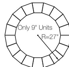
To enlarge the radius for planters and walls, simply 'gap' the back to make the desired radius. (You will not see the gaps because they are against the backfill.) Be sure to use filter fabric between the wall and the backfill. (See Tech Guide for complete instructions.)
