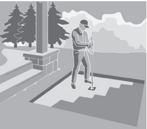
STEP 2: EXCAVATE, FLATTEN, AND COMPACT BASE AT APPROXIMATE 5" DEPTH
